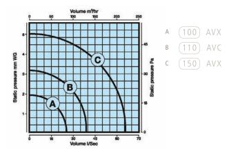
LIGHT RATING/OUTPUT: 12V AC ~50Hz; INPUT: 220/240 V ~50Hz, IP24; □ ▲; MAXIMUM PRESSURE: AVX100: 20pa, AVC110: 120pa, AVX150: 50pa; FAN SPEED: 2400rpm, AVC 1400rpm; TIMER: adjustable 1-20 mins; construction: moulded high temperature VO rated thermoplastic; BULB: GU5.3 35W Dichroic; MOTOR: Single phased induction motor with pre-oiled bearings. Thermal overload protection; MAX OPERATING TEMP: 40°C; AVCPRO120CDFSLC 60°C. CE
