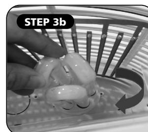
*NOTE: if the Insect Killer is free-standing, remove the collection tray and turn the unit upside down to gain access to the lamps.*
