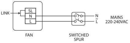
Fig. 2 Continuous Boost (15 L/s) with no trickle facility. Note:- Link must be fitted between Live & Switched Live terminals.
